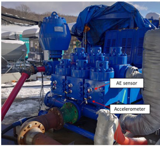
Fig. 4—Sensor deployed and damaged swab in Field Test 3: (left) sensor deployment on Pump 1 and (right) damaged swab from Pump 2.
