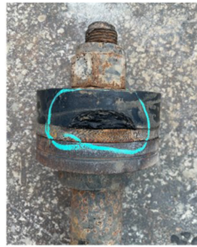
Fig. 4—Sensor deployed and damaged swab in Field Test 3: (left) sensor deployment on Pump 1 and (right) damaged swab from Pump 2.
